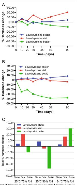
**Fig. 2** Hardness change of levothyroxine tablets. **A** Percent hardness change over time: 25 °C/75% RH. **B** Percent hardness change over time: 25 °C/90% RH. **C** Total percent hardness change under 90-day patient use or 2-day shipping conditions. Abbreviation: RH, relative humidity
