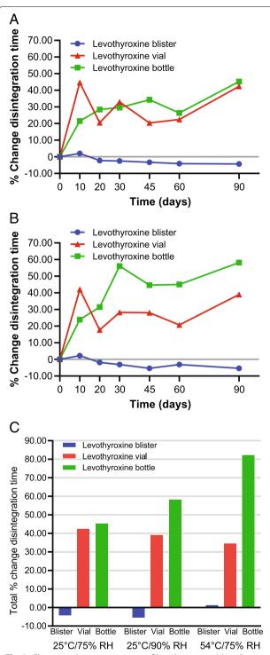
**Fig. 3** Change in disintegration time of levothyroxine tablets. **A** Percent change in disintegration time: 25 °C/75% RH. **B** Percent change in disintegration time: 25 °C/90% RH. **C** Total percent change in disintegration time under 90-day patient use or 2-day shipping conditions. Abbreviation: RH, relative humidity
