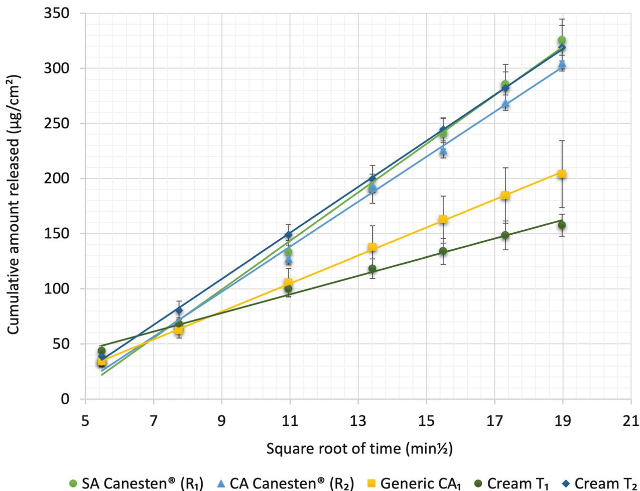
**Fig. 3** Release rate profiles from SA and CA Canesten® 1% CLZ (R<sub>1</sub> and R<sub>2</sub>), CA-marketed 1% CLZ generic cream (CA<sub>1</sub>), and extemporaneously compounded creams T<sub>1</sub> and T<sub>2</sub> (n=6)
