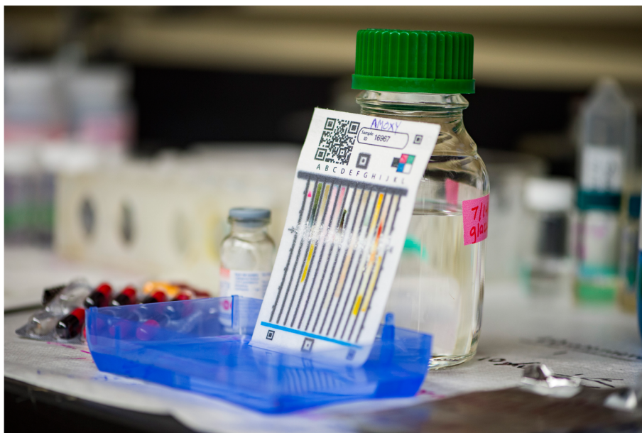
Fig. 4 Paper analytical device running a sample. Source: Barbara Johnson/University of Notre Dame, permission granted by Marya Lieberman, University of Notre Dame
